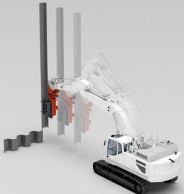
Horizontal movement with a stationary excavator.
