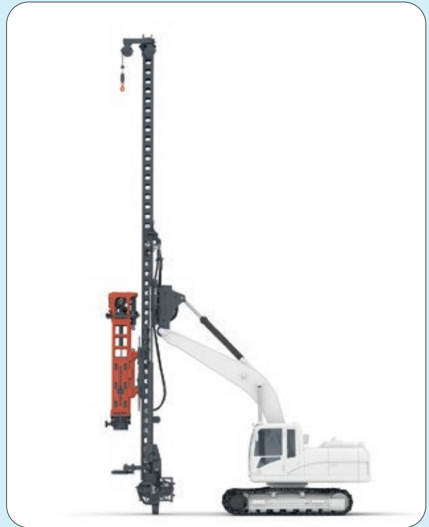
MOVAX multi-tool piling leader-mounted
